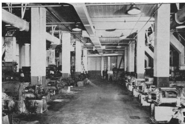
Fig. 14. Pre-pressing flaxseed on mechanical screw presses.
